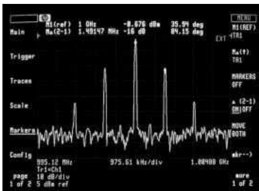
Measure phase of sidebands; determine whether AM or FM.
